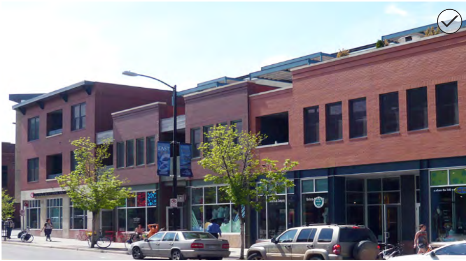
Where a new structure must exceed a traditional building width, break the façade into modules that suggest traditional building widths.
