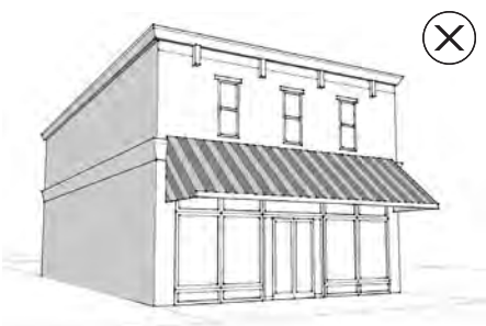
Awnings should not obscure the frame and details of a building. Solid colored awnings should be used rather than striped awnings.
