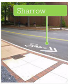
Sharrows – Street marking indicated a travel lane that is to be 'shared' by both bicycle and vehicular traffic
