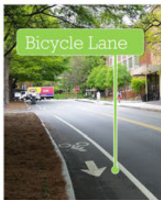
Bicycle Lanes – Bicycle lanes are areas of the roadway dedicated for bicycle-only traffic. The bike lane is designated through pavement markings and signage. These lanes are typically 4 feet to 7 feet wide, located on the right side of the roadway, and are used in the same direction as vehicular traffic.
