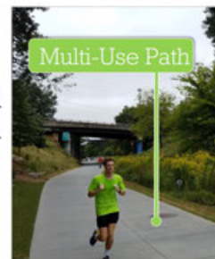
Multi-Use Paths – Trails and pathways designated for use by both pedestrians and bicyclists with a typical width between 10 and 12 feet.
