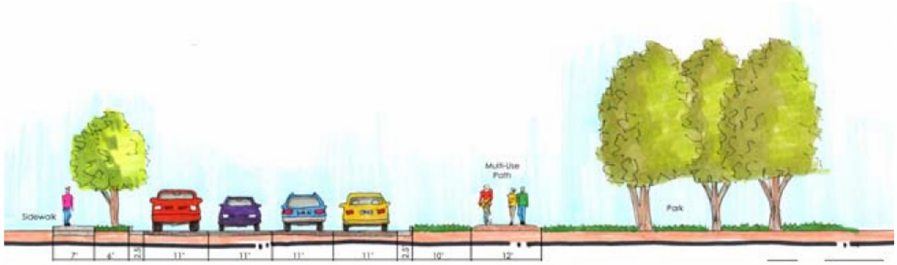
Figure 5.5: Possible cross-section for Atlanta Street between Azalea / Riverside Drive and the Allenbrook Roundabout (Alternative 2)
